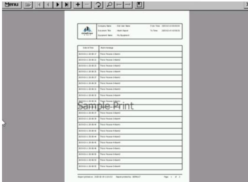
You can zoom/scroll the report using the finger tap on the HMI screen. Close the pdf file using the 'Menu→Exit' option available at the pdf viewer menu bar.
